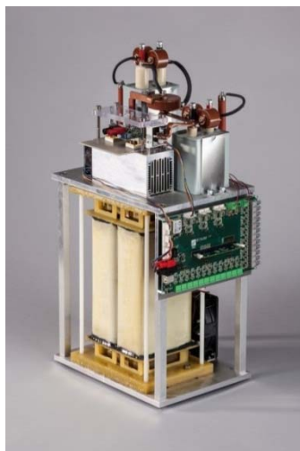
Figure 4-6: Left: Medium-voltage DC / DC converter, Right: Efficiency of the converter
